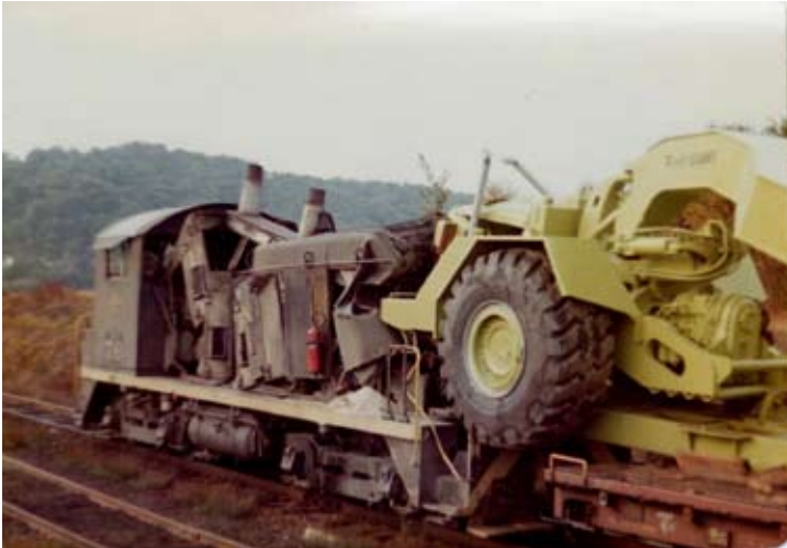
A runaway flat car with an earth mover aboard collided with engine 76. Note the impression of the earth mover's front bumper in 76's body and radiator. Charles A. Ross photo
